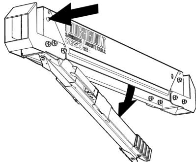
**2** Push down leg brace till it is fully locked out. Verify that the top of the legs lock solidly against the body.
